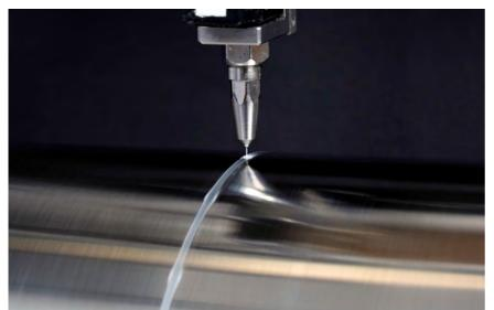
The new VINNAPAS<sup>®</sup> EP 6420 offers best-in-class performance for nozzle applications, showing excellent running stability without skin formation. This makes the VAE binder ideal for formulating water-based adhesives in demanding paper and packaging applications (photo: Wacker Chemie AG).
